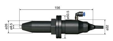
Specifications... • Piezoelectric Transducer : Bolt-Clamped PZT Type
