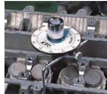
2. Set angle torque gauge and fix it with L-stopper or flexible stopper.
