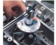
4. Fasten gauge to specified angle with spinner handle.
